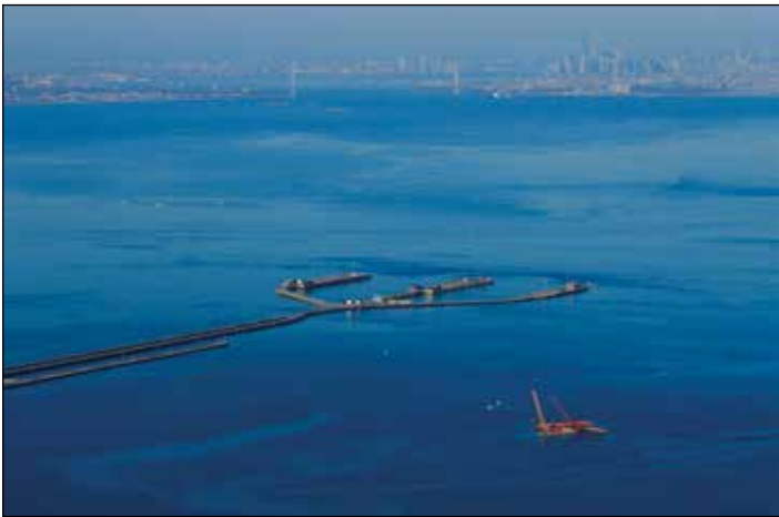
J.T. Cleary's dewatering station, lower right, was a large anchor with a single-point mooring. The dewatering site at times had a half-dozen barges waiting for the water to clarify sufficiently for decanting. The pier to Naval Weapons Station Earle is in mid-photo, and the city of Manhattan in the background.
